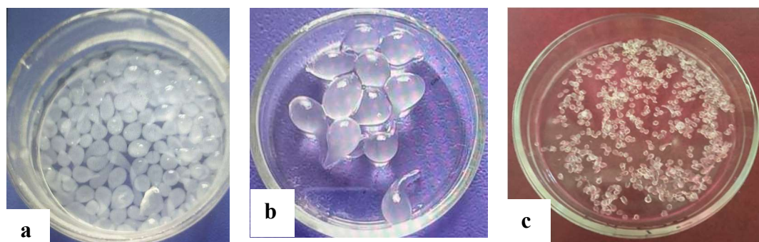
Fig.1. Changes in the size of hydrogel beads based on calcium-alginate and laponite ( C_{alg}=2\% , C_{lap}=0.5\% , C_{CaCl_2}=0.5\% ) during processing (a-after synthesis; b-after swelling; c-after drying)
